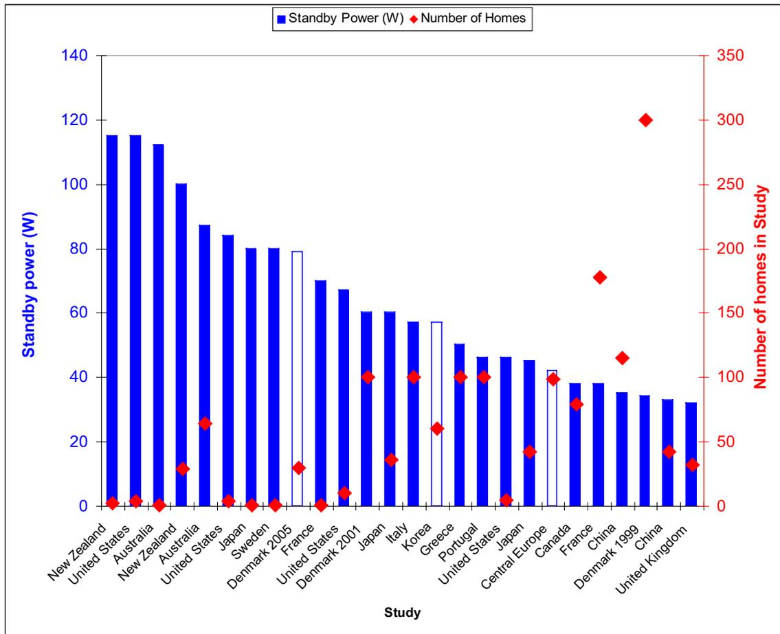
Figure 3. Summary of measurements of standby power consumption in homes. Adapted from Meier (2002) with new data shown as unfilled bars.
